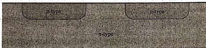
Figure 1.12 Selected regions of the wafer have been changed to p -type material by exposure to impurities in a diffusion furnace.
