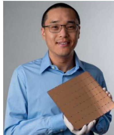
CERABRAS, 400'000 Cores (0.016 \mu\text{m} ) 46'225 mm 2 → WAFER-SCALE CEREBRAS CS-1 (09/2019 → 2.5 M$)
