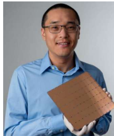
CERABRAS, 400'000 Cores (0.016 µm) 46'225 mm² → WAFER-SCALE CEREBRAS CS-1 (09/2019 → 2.5 M$)
